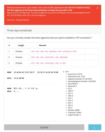
Figure 2: Students learn the TCP three-way handshake by reordering packets.
